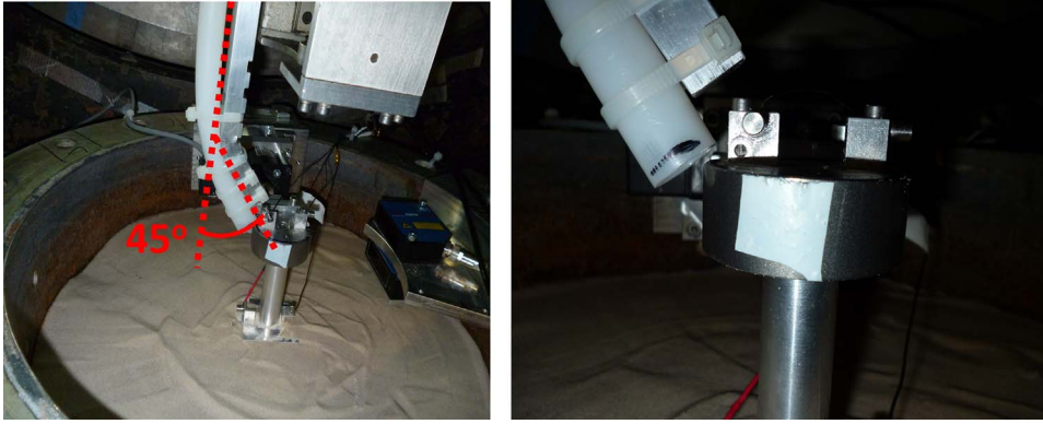
Fig. 4. Left: The shooting tube is attached on the actuator arm, right: the lower edge of the tube targets on the head of the structure with an angle of 45°.
